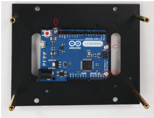
Figure 4-22. Arduino board mounted using three spacers
