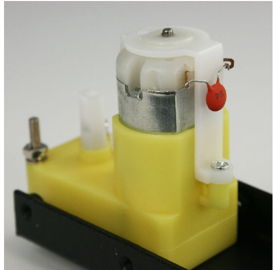
Figure 4-11. Crimp the capacitor leads to the motor terminals
