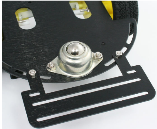
Figure 3-9. Sensor bracket viewed with the robot upside down
