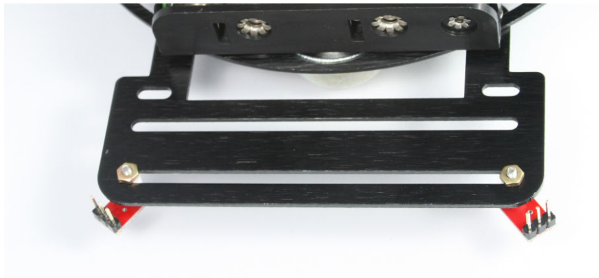
Figure 3-27. Reflectance Sensor location for Edge Detection
