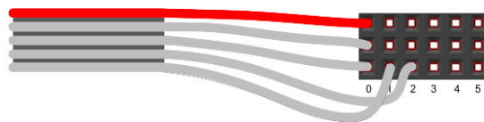
Figure 2-13. Ribbon cable connections to shield pins
