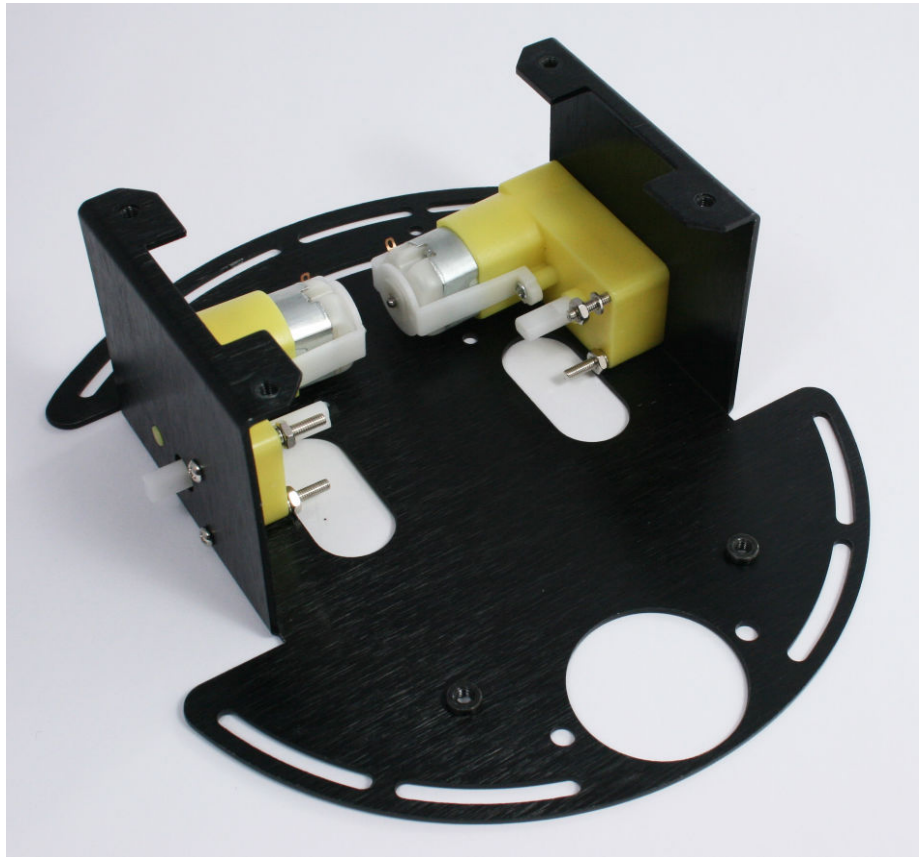
Figure 3-4. Motors mounted on the chassis lower plate
