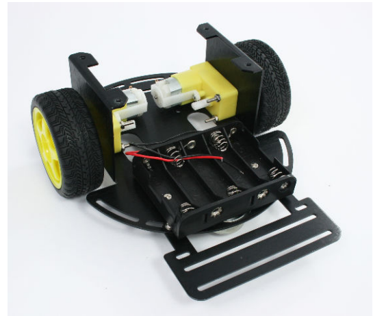
Figure 3-11. Chassis with Battery Pack Attached
